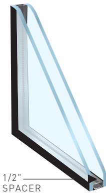
1" VE1-48 INSULATING 1/4" (6mm) clear with VE-48 #2 1/2" (13.2mm) airspace 1/4" (6mm) clear
